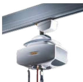
4 GH2 F Flexible ceiling hoist that can be moved from one rail system to another. It installs and removes itself from the rail system automatically. Max lifting capacity 200 kg . . . 120001-xxxx Note: Can also be used in the GH3 rails.
