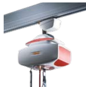
5 GH2 F HD Heavy duty flexible ceiling hoist. Can be moved from one rail system to another. It installs and removes itself from the rail system automatically. Max lifting capacity 250 kg . . . 120001-xxxx Note: Can also be used in the GH3 rails.
